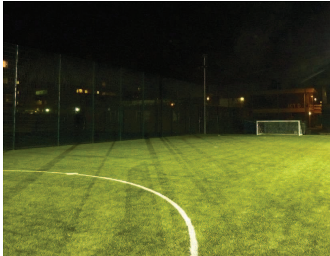
3g five-a-side pitch at 200 lux lighting level
